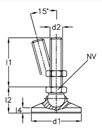
A/F = 24 d1 = 60 d2 = 16 l1 = 125 l2 = l4 = -Static load (N) = 30 Weight in (g) = 545
